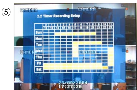
Setup Date & Time Schedule in the Same Way. After Finishing Schedule Setup, Press 'Return' for Save & Exit
